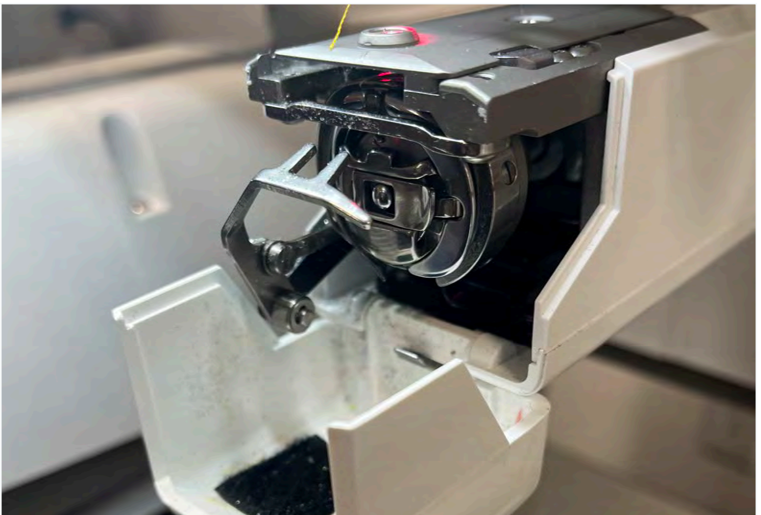
Figure 12: Insert the bobbin case into the rotary hook and secure it with a click.
