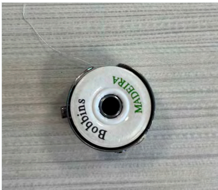
Figure 10: The bobbin inserted into the bobbin case in the clockwise direction.
