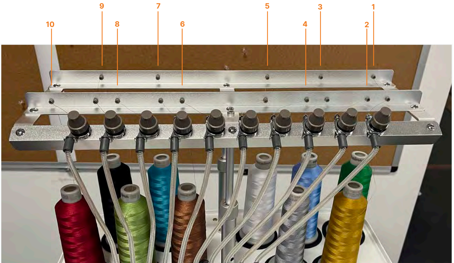
Figure 13: Pass the thread through the thread path located in the front and back of the metal thread rack. (Needle paths 1, 3, 5, 7, and 9 have a back and front needle path. Needles 2, 4, 6, 8, 10 only have a front needle path).
