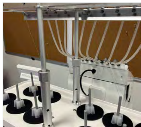
Figure 5: Back view of the thread rack indicating where it attaches to the thread stand.
