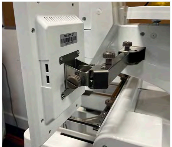
Figure 9: Adjust the touch screen panel arm to your preferred position for easy access and visibility during operation.
