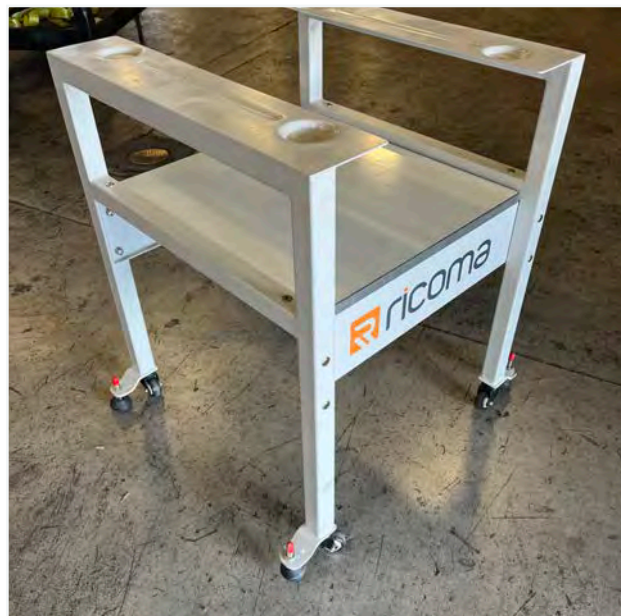
Figure 1: Embroidery machine steel stand put together
