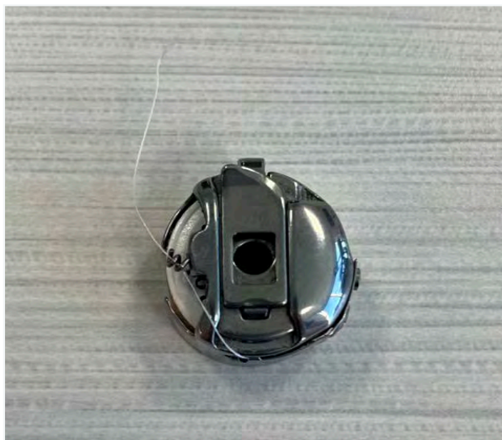
Figure 11: The bobbin thread wrapped around the pigtail twice.
